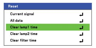
A confirmation box is displayed. Select **OK** using ◀ or ▶ and press ◀ to reset the selected Lamp hours to zero.
